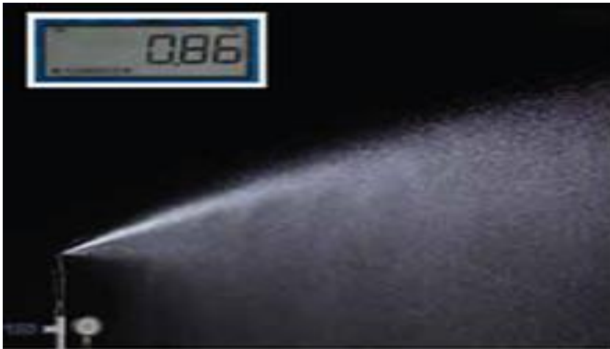
1800 Spray with PRS at 79 psi inlet pressure. PRS regulates flow to 0.86 gallons per minute.
